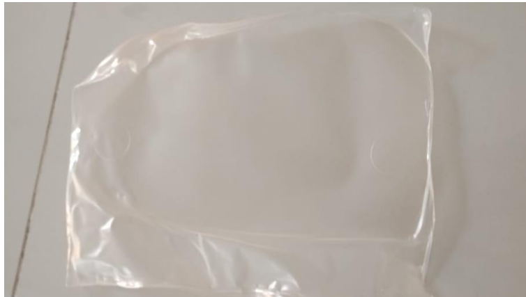
Figure 2. Edible Film from banana hump starch with the addition of polyethylene glycol and carrageenan
