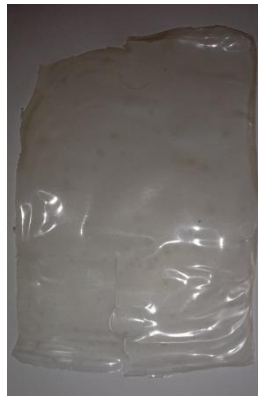
Picture2. Edible Film from jackfruit seed starch with the addition of chitosan
