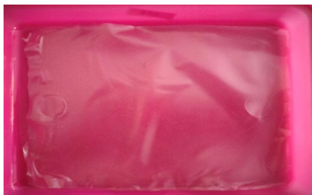
Fig. 2 breadfruit starch edible film with the addition of carrageenan
